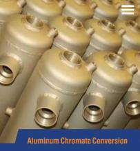
This coating increases the adhesion of paint to the metal surface and increases the resistance to metal corrosion and is used to create a chromate coating on aluminum and galvanized surfaces.
