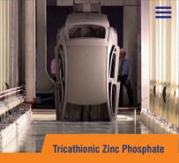
This coating are two kinds of "Zn-Ni-Ca" and "Zn-Ni-Mn". They have different applications in various industries and diversify from rough heavy crystals to microscopic soft crystals. Their colors are light gray to dark gray. In splash method, coating thickness shall be 2 to 5 microns and 2 to 10 microns in impression method.
