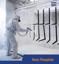
This coating will be used for crystalizing of metal parts to protect against environmental corrosion and surface preparation for paint stability and more adhesion completely.
