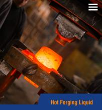
Hot forging liquid is water-soluble liquid and prevents adhesion by creating a white layer between the part and the mold with no environmental pollution. Also this liquid prevents damage to the mold by temperature resistance up to 1200 degrees Celsius.
