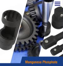
This kind of phosphate will be applied in shape of immersion only and their color is blackish gray. The required time of coating is varied between 15 to 30 minutes and coating thickness amount on metal surface shall be 5 to 20 microns.
