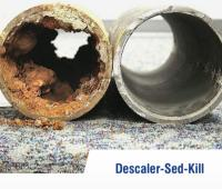
Descalers are based on acidic or neutral compounds, which are used to remove any carbonate deposits, iron oxide, iron hydroxide, and iron phosphate.
